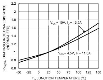
Figure 6. On-Resistance Variation with Junction
