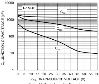
Figure 10. Typical Junction Capacitance
