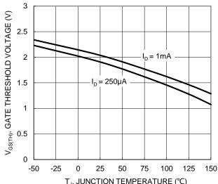
T<sub>J</sub>, JUNCTION TEMPERATURE (°C) Figure 8. Gate Threshold Variation vs. Junction Temperature
