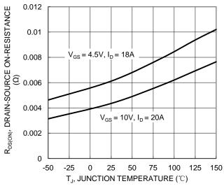
Figure 7. On-Resistance Variation with Temperature
