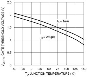
Figure 8. Gate Threshold Variation vs. Temperature
