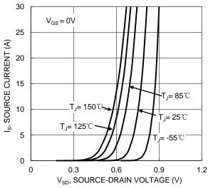
Figure 9. Diode Forward Voltage vs. Current
