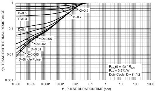
Figure 13. Transient Thermal Resistance
