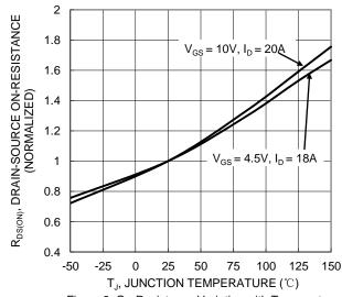
Figure 6. On-Resistance Variation with Temperature
