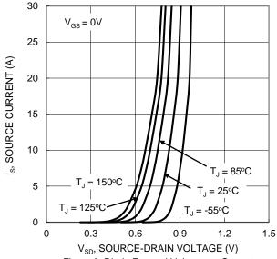
Figure 9. Diode Forward Voltage vs. Current
