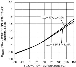
Figure 6. On-Resistance Variation with Junction Temperature
