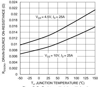
Figure 7. On-Resistance Variation with Junction Temperature
