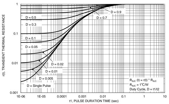
Figure 13 Transient Thermal Resistance
