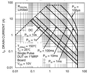
V<sub>DS</sub>, DRAIN-SOURCE VOLTAGE (V) Figure 12. SOA, Safe Operation Area
