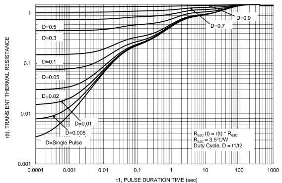
Figure 13. Transient Thermal Resistance
