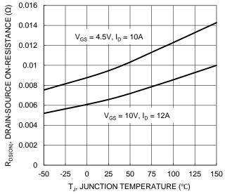
Figure 7. On-Resistance Variation with Temperature
