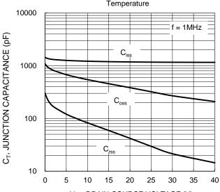
$V_{\rm DS}$ , DRAIN-SOURCE VOLTAGE (V) Figure 10. Typical Junction Capacitance
