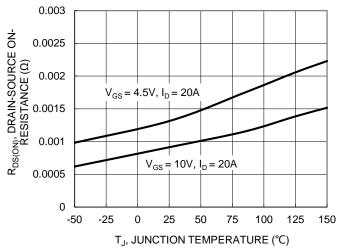
Figure 7. On-Resistance Variation with Temperature
