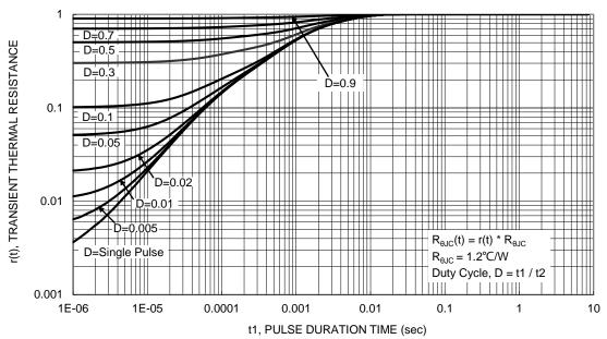
Figure 13. Transient Thermal Resistance
