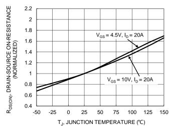
Figure 6. On-Resistance Variation with Temperature
