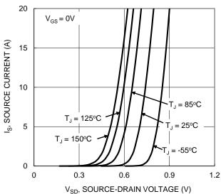
Figure 9. Diode Forward Voltage vs. Current
