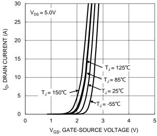
Figure 2. Typical Transfer Characteristic
