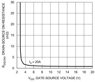
Figure 4. Typical Transfer Characteristic
