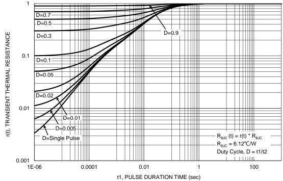
Figure 13. Transient Thermal Resistance
