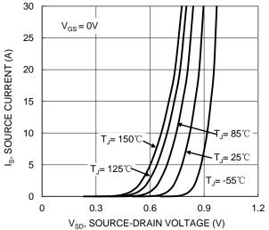
Figure 9. Diode Forward Voltage vs. Current
