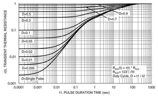
Figure 14. Transient Thermal Resistance
