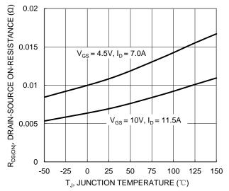
Figure 7. On-Resistance Variation with Temperature
