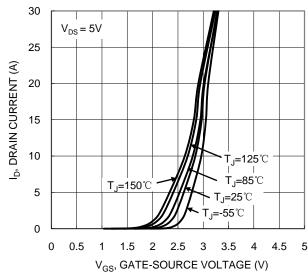
Figure 2. Typical Transfer Characteristic
