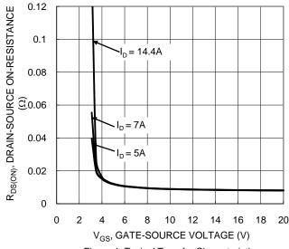
Figure 4. Typical Transfer Characteristic
