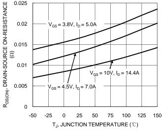
Figure 7. On-Resistance Variation with Temperature
