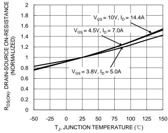
Figure 6. On-Resistance Variation with Temperature
