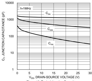
Figure 10. Typical Junction Capacitance
