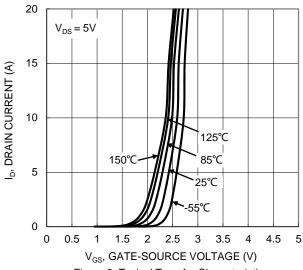
Figure 2. Typical Transfer Characteristic
