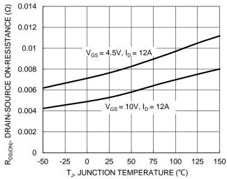
Figure 7. On-Resistance Variation with Temperature
