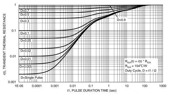
Figure 13. Transient Thermal Resistance
