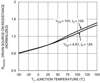
Figure 6. On-Resistance Variation with Temperature
