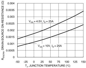
Figure 7. On-Resistance Variation with Temperature
