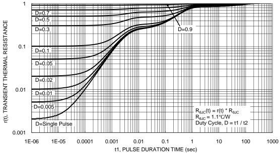
Figure 13. Transient Thermal Resistance
