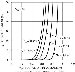
Figure 9. Diode Forward Voltage vs. Current
