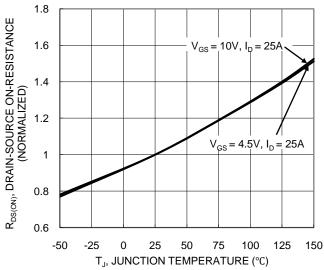
Figure 6. On-Resistance Variation with Temperature
