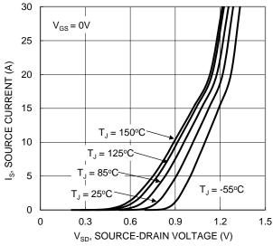
Figure 9. Diode Forward Voltage vs. Current
