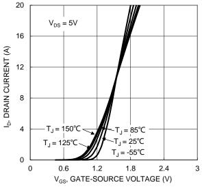
Figure 2. Typical Transfer Characteristic
