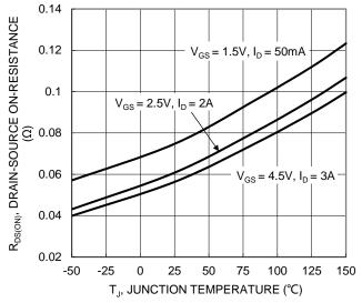
Figure 7. On-Resistance Variation with Temperature
