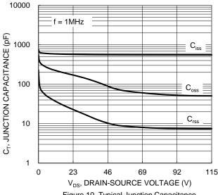
Figure 10. Typical Junction Capacitance
