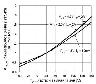
Figure 6. On-Resistance Variation with Temperature
