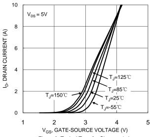
Figure 2. Typical Transfer Characteristic
