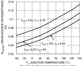
Figure 7. On-Resistance Variation with Junction Temperature
