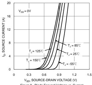
Figure 9. Diode Forward Voltage vs. Current
