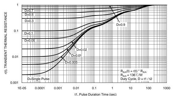
Figure 13. Transient Thermal Resistance
