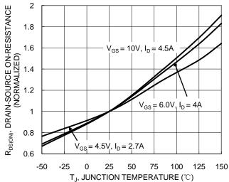
Figure 6. On-Resistance Variation with Junction Temperature
