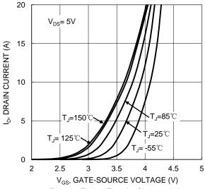
Figure 2. Typical Transfer Characteristic
