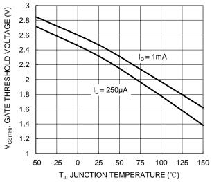
Figure 8. Gate Threshold Variation vs. JunctionTemperature
