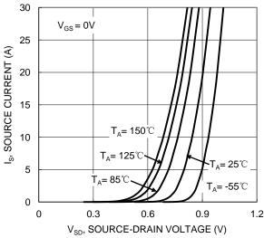
Figure 9. Diode Forward Voltage vs. Current
