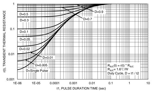
Figure 13. Transient Thermal Resistance
