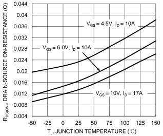
Figure 7. On-Resistance Variation with Temperature
