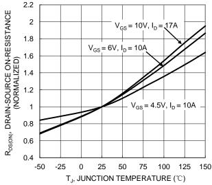
Figure 6. On-Resistance Variation with Temperature
