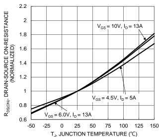
Figure 6. On-Resistance Variation with Junction Temperature
