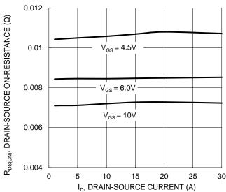
Figure 3. Typical On-Resistance vs. Drain Current and
