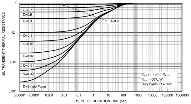
Figure 13. Transient Thermal Resistance
