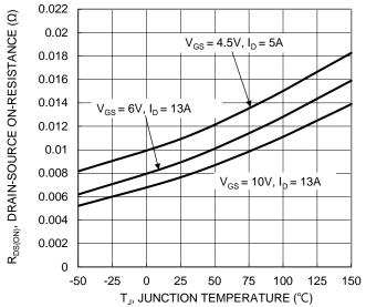
Figure 7. On-Resistance Variation with Junction Temperature
