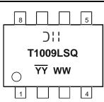
$\bigcirc$  | | = Manufacturer's Marking T1009LSQ = Product Type Marking Code  $\underline{YYWW}$  = Date Code Marking  $\overline{YY}$  = Year (ex: 23 = 2023) WW = Week (01 to 53)
