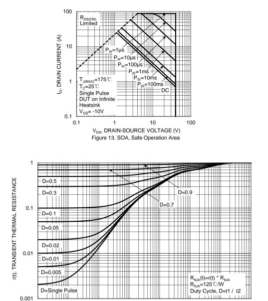
t1, PULSE DURATION TIME (sec) Figure 14. Transient Thermal Resistance
