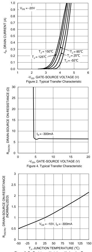
Figure 6. On-Resistance Variation with Junction Temperature
