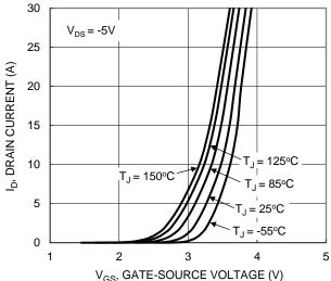
Figure 2. Typical Transfer Characteristic
