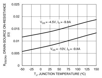
Figure 7. On-Resistance Variation with Temperature
