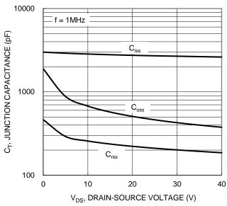
Figure 10. Typical Junction Capacitance
