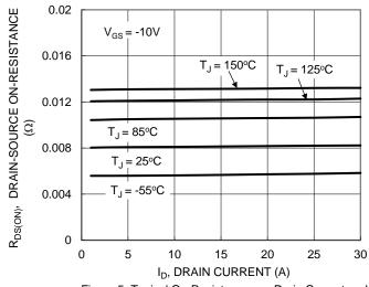
Figure 5. Typical On-Resistance vs. Drain Current and Temperature
