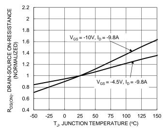
Figure 6. On-Resistance Variation with Temperature
