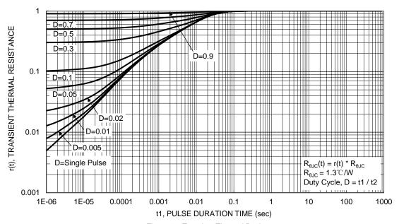
Figure 13. Transient Thermal Resistance
