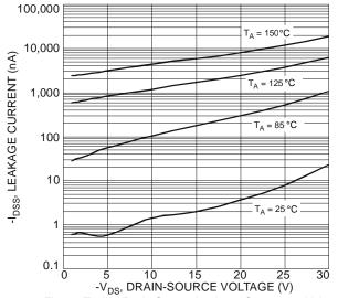
Fig. 13 Typical Drain-Source Leakage Current vs. Voltage
