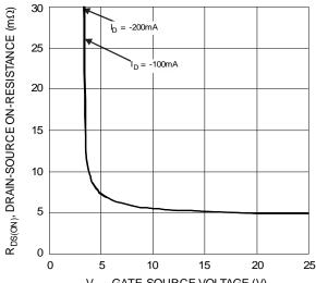
V<sub>GS</sub> GATE-SOURCE VOLTAGE (V) Figure 4 Typical Drain-Source On-Resistance vs. Gate-Source Voltage
