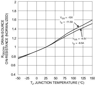
Figure 6 On-Resistance Variation with Temperature
