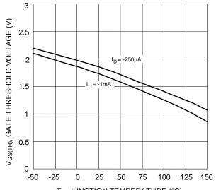
$\label{eq:total_total} T_J, \, \text{JUNCTION TEMPERATURE (°C)}$  Figure 8 Gate Threshold Variation vs. Junction Temperature
