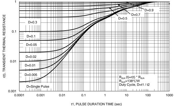
Figure 13. Transient Thermal Resistance
