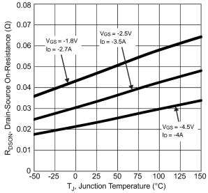
Fig. 7 On-Resistance Variation with Junction Temperature
