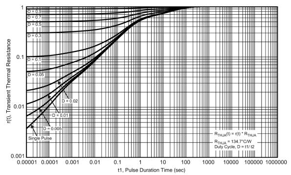
Fig. 13 Transient Thermal Resistance
