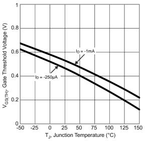
Fig. 8 Gate Threshold Variation vs Junction Temperature
