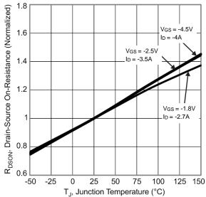
Fig. 6 On-Resistance Variation with Junction Temperature
