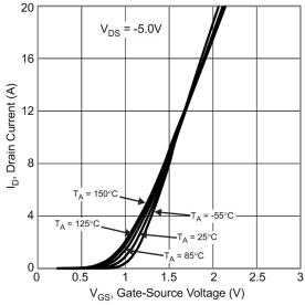
Fig. 2 Typical Transfer Characteristic
