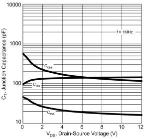
Fig. 10 Typical Junction Capacitance
