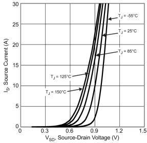
Fig. 9 Diode Forward Voltage vs Current
