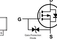
Pin Configuration Internal Schematic
