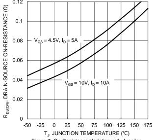
Figure 7. On-Resistance Variation with Junction Temperature
