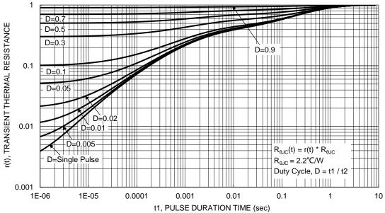
Figure 13. Transient Thermal Resistance
