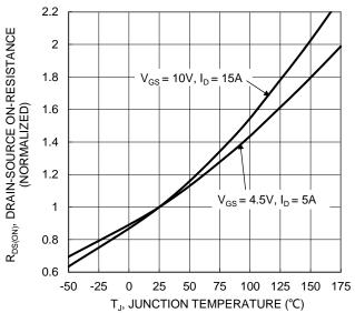
Figure 6. On-Resistance Variation with Junction Temperature
