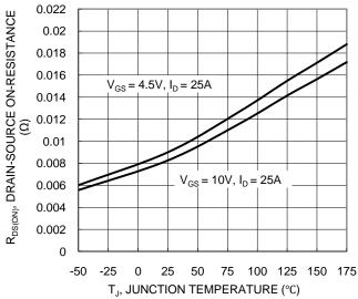
Figure 7. On-Resistance Variation with Temperature
