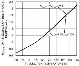
Figure 6. On-Resistance Variation with Temperature
