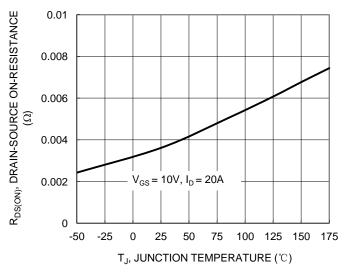
Figure 7. On-Resistance Variation with Temperature
