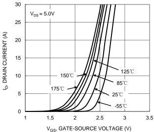
Figure 2. Typical Transfer Characteristic
