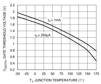
Figure 8.Gate Threshold Variation vs. Junction Temperature
