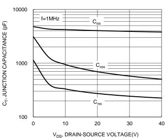
Figure 10. Typical Junction Capacitance
