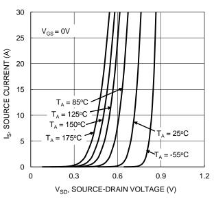
Figure 9. Diode Forward Voltage vs. Current
