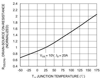
Figure 6. On-Resistance Variation with Temperature
