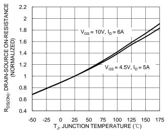
Figure 6.On-Resistance Variation with Temperature
