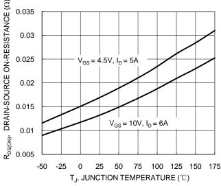
Figure 7. On-Resistance Variation with Temperature
