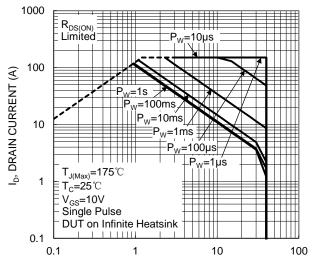
V<sub>DS</sub>, DRAIN-SOURCE VOLTAGE (V) Figure 13. SOA, Safe Operation Area
