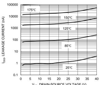
V<sub>DS</sub>, DRAIN-SOURCE VOLTAGE (V) Figure 10. Typical Drain-Source Leakge Current vs Voltage
