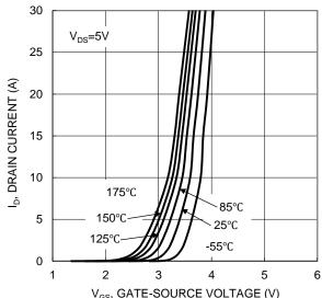
$V_{GS}$ , GATE-SOURCE VOLTAGE (V) Figure 2. Typical Transfer Characteristic
