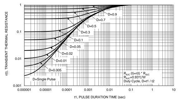
Figure 14. Transient Thermal Resistance
