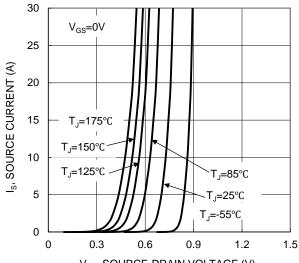
$V_{\text{SD}}$ , SOURCE-DRAIN VOLTAGE (V) Figure 9. Diode Forward Voltage vs Current
