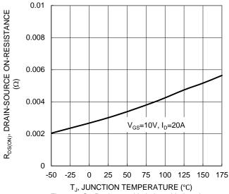
Figure 7. On-Resistance Variation with Junction Temperature
