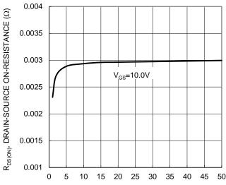
I<sub>D</sub>, DRAIN-SOURCE CURRENT (A) Figure 3. Typical On-Resistance vs Drain Current and Gate Voltage
