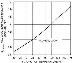
Figure 6. On-Resistance Variation with Junction Temperature
