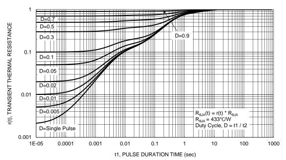
Figure 13. Transient Thermal Resistance
