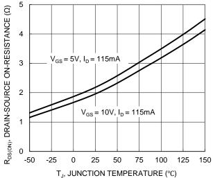
Figure 7. On-Resistance Variation with Junction Temperature
