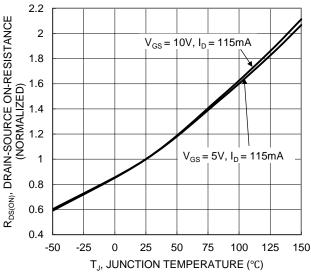
Figure 6. On-Resistance Variation with Junction Temperature
