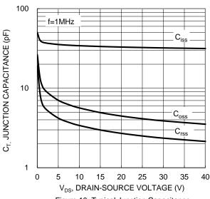
Figure 10. Typical Junction Capacitance
