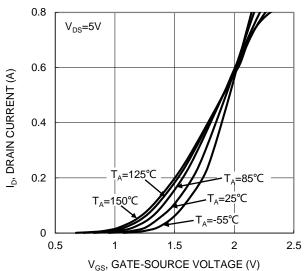
Figure 2. Typical Transfer Characteristic
