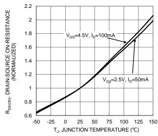
Figure 6. On-Resistance Variation with Junction Temperature
