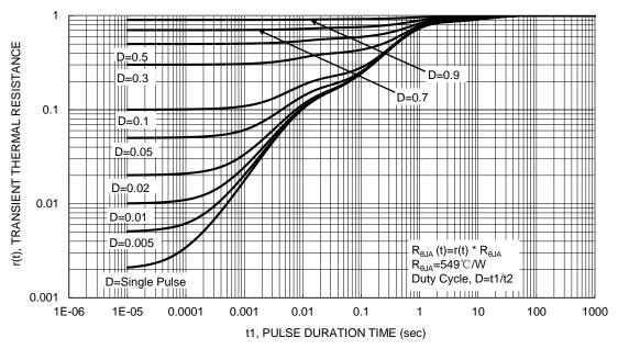
Figure 13. Transient Thermal Resistance
