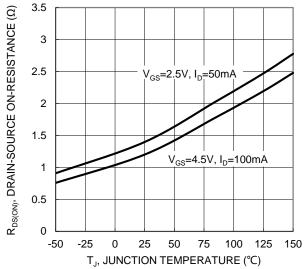
Figure 7. On-Resistance Variation with Junction Temperature
