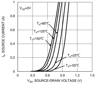
Figure 9. Diode Forward Voltage vs. Current
