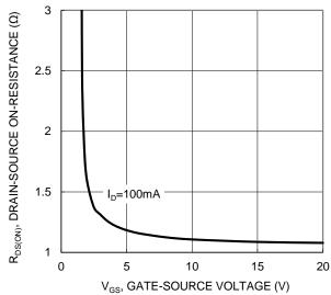
Figure 4. Typical Transfer Characteristic
