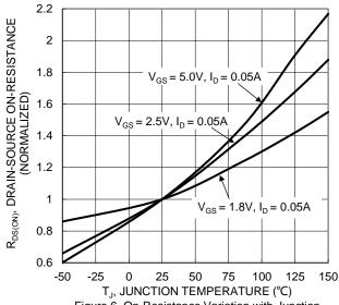
Figure 6. On-Resistance Variation with Junction Temperature
