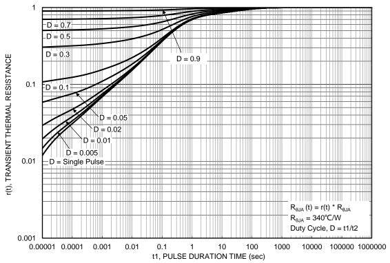
Figure 13. Transient Thermal Resistance
