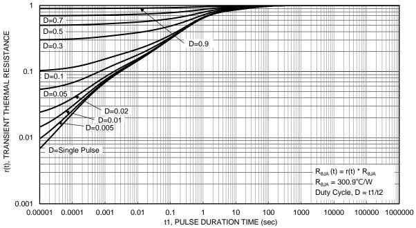
Figure 13. Transient Thermal Resistance
