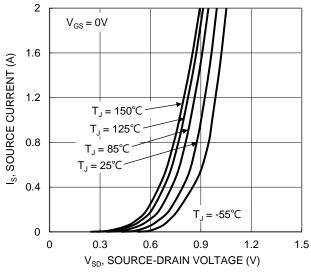
Figure 9. Diode Forward Voltage vs. Current
