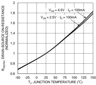
Figure 6. On-Resistance Variation with Junction Temperature
