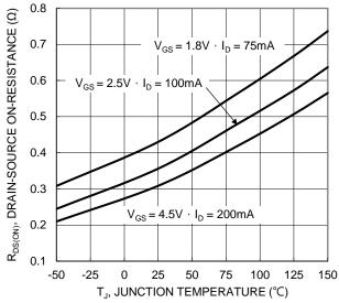
Figure 7. On-Resistance Variation with Junction Temperature
