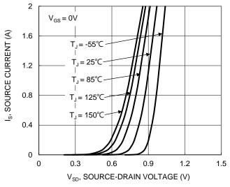
Figure 9. Diode Forward Voltage vs. Current
