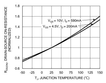
Figure 6. On-Resistance Variation with Junction Temperature
