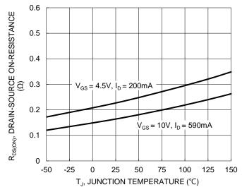
Figure 7. On-Resistance Variation with Junction Temperature
