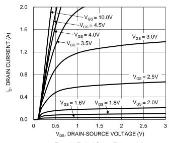
Figure 1. Typical Output Characteristic
