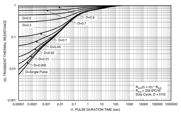
Figure 13. Transient Thermal Resistance
