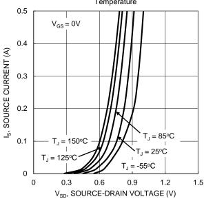
Figure 9. Diode Forward Voltage vs. Current
