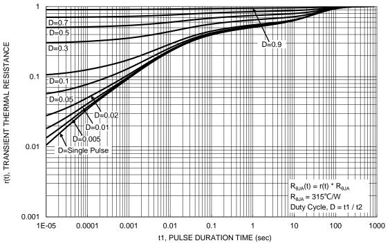
Figure 13. Transient Thermal Resistance
