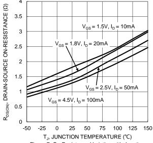
Figure 7. On-Resistance Variation with Junction Temperature
