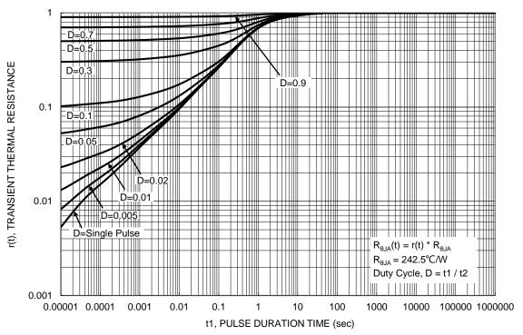
Figure 13. Transient Thermal Resistance
