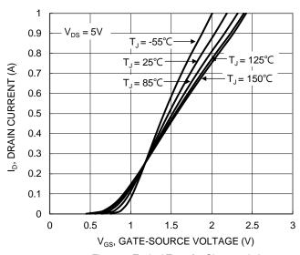
Figure 2. Typical Transfer Characteristic
