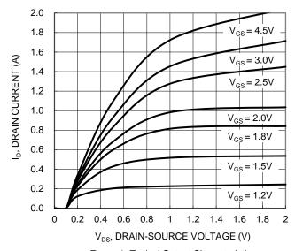
Figure 1. Typical Output Characteristic
