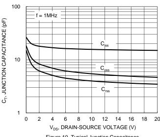
Figure 10. Typical Junction Capacitance
