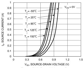
Figure 9. Diode Forward Voltage vs. Current
