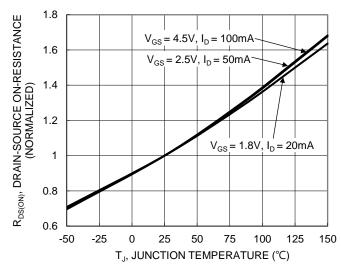
Figure 6. On-Resistance Variation with Junction Temperature
