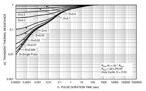
Figure 13. Transient Thermal Resistance
