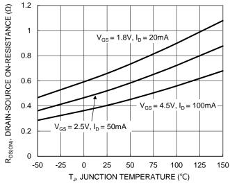
Figure 7. On-Resistance Variation with Junction Temperature
