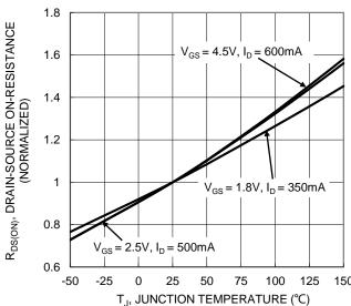
Figure 6. On-Resistance Variation with Junction Temperature
