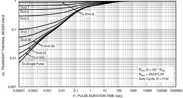
Figure 13. Transient Thermal Resistance
