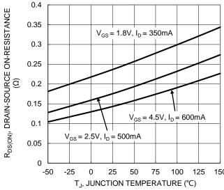
Figure 7. On-Resistance Variation with Junction Temperature
