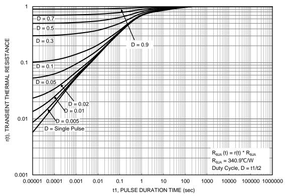
Figure 13. Transient Thermal Resistance
