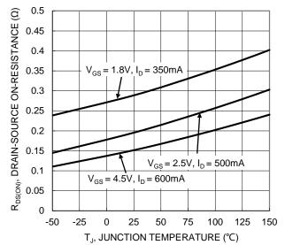
Figure 7. On-Resistance Variation with Junction Temperature
