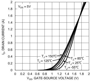
Figure 2. Typical Transfer Characteristic
