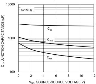
Figure 10. Typical Junction Capacitance
