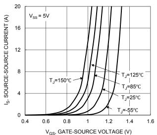
Figure 2. Typical Transfer Characteristic
