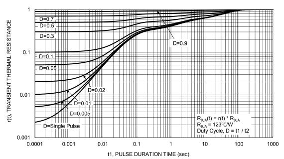
Figure 13. Transient Thermal Resistance
