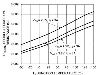
Figure 7. On-Resistance Variation with Junction Temperature
