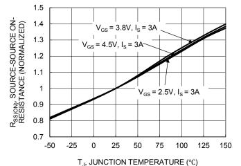
Figure 6. On-Resistance Variation with Junction Temperature
