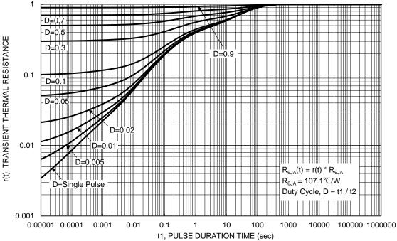
Figure 13. Transient Thermal Resistance
