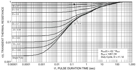
Figure 11 Transient Thermal Resistance
