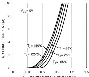
V<sub>SD</sub>, SOURCE-DRAIN VOLTAGE (V) Figure 9. Diode Forward Voltage vs. Current
