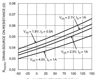
T<sub>J</sub>, JUNCTION TEMPERATURE (°C) Figure 7. On-Resistance Variation with Junction Temperature
