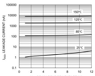
$\rm V_{DS},$  DRAIN-SOURCE VOLTAGE (V) Figure 10. Typical Drain-Source Leakage Current vs. Voltage
