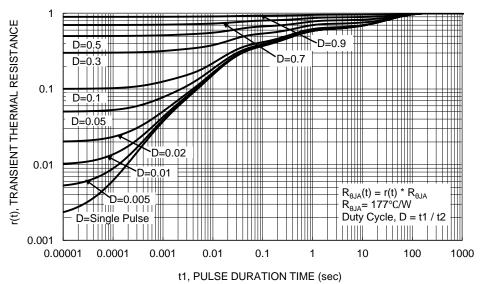
Figure 14. Transient Thermal Resistance
