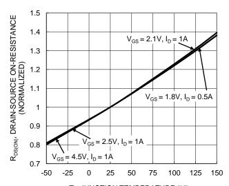
T<sub>J</sub>, JUNCTION TEMPERATURE (°C) Figure 6. On-Resistance Variation with Junction Temperature
