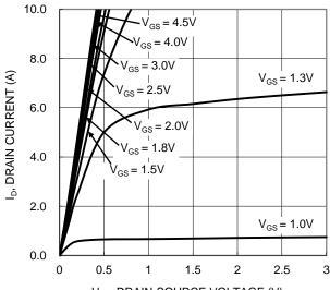
V<sub>DS</sub>, DRAIN-SOURCE VOLTAGE (V) Figure 1. Typical Output Characteristic
