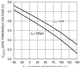
T<sub>J</sub>, JUNCTION TEMPERATURE (°C) Figure 8. Gate Threshold Variation vs. Junction Temperature
