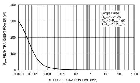
Figure 13. Single Pulse Maximum Power Dissipation
