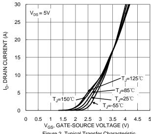
Figure 2. Typical Transfer Characteristic
