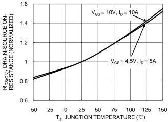
Figure 6. On-Resistance Variation with Temperature
