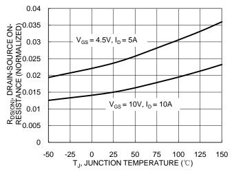
Figure 7. On-Resistance Variation with Temperature
