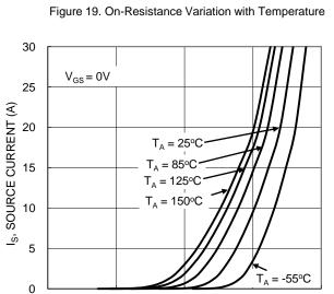
V<sub>SD</sub>, SOURCE-DRAIN VOLTAGE (V) Figure 21. Diode Forward Voltage vs. Current
