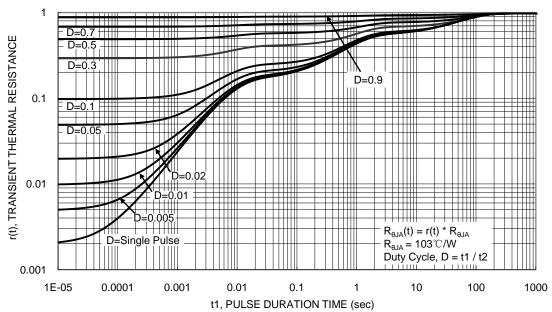
Figure 25. Transient Thermal Resistance
