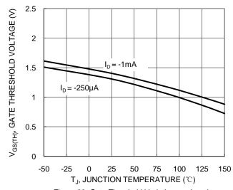
Figure 20. Gate Threshold Variation vs. Junction Temperature
