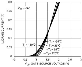
Figure 15. Typical Transfer Characteristic
