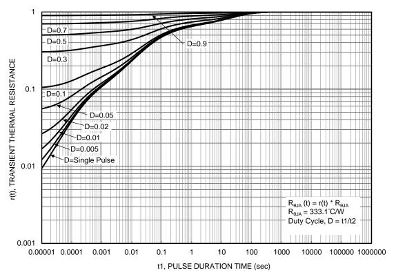
Figure 13. Transient Thermal Resistance
