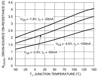
Figure 20. On-Resistance Variation with Junction Temperature
