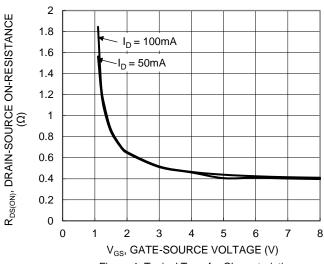
Figure 4. Typical Transfer Characteristic
