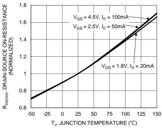
Figure 6. On-Resistance Variation with Junction Temperature
