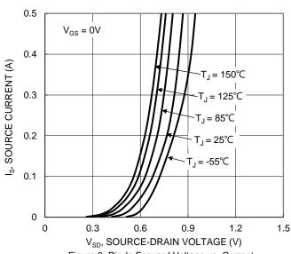
Figure 9. Diode Forward Voltage vs. Current
