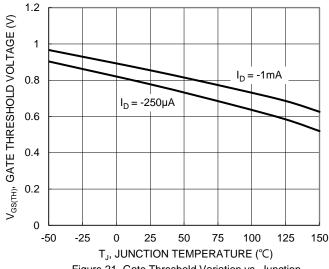
Figure 21. Gate Threshold Variation vs. Junction Temperature
