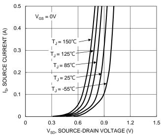
Figure 22. Diode Forward Voltage vs. Current
