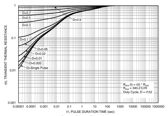
Figure 26. Transient Thermal Resistance
