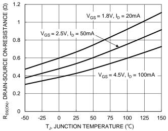
Figure 7. On-Resistance Variation with Junction Temperature
