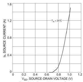
Fig. 8 Diode Forward Voltage vs. Current
