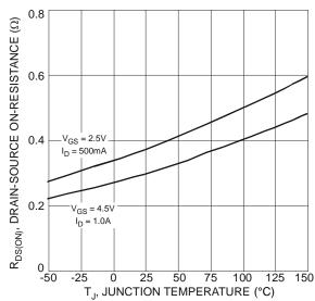
Fig. 6 On-Resistance Variation with Temperature
