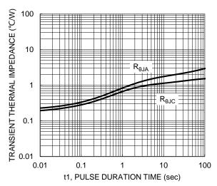
Fig. 5 Typical Transient Thermal Impedance
