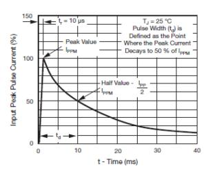
Fig. 3 - Pulse Waveform
