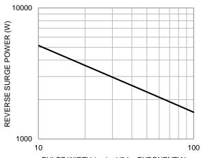
PULSE WIDTH (ms) - 1/2 I<sub>PP</sub> EXPONENTIAL WAVEFORM Fig. 4 Reverse Power Capability
