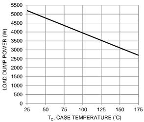
Fig. 2 Load Dump Power Characteristics (10ms Exponential Waveform)
