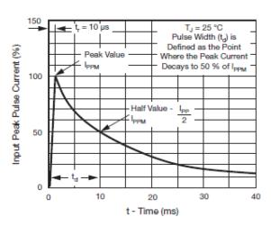
Fig. 3 - Pulse Waveform
