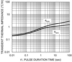
Fig. 5 Typical Transient Thermal Impedance
