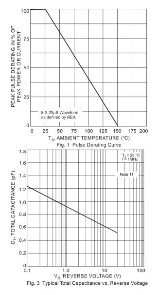
Note: 11. Measured from line to be protected to ground pin.
