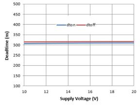
Figure 23. Deadtime vs. Supply Voltage
