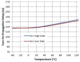
Figure 4. Turn-on Propagation Delay vs. Temperature
