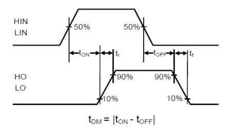
Figure 1. Switching Time Waveform Definitions
