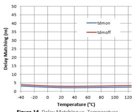
Figure 14. Delay Matching vs. Temperature
