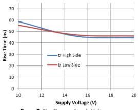
Figure 7. Rise Time vs. Supply Voltage
