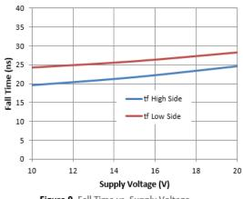
Figure 9. Fall Time vs. Supply Voltage
