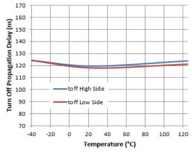
Figure 6. Turn-off Propagation Delay vs. Temperature
