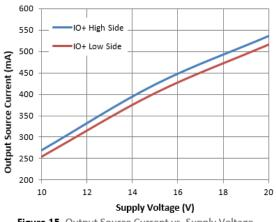
Figure 15. Output Source Current vs. Supply Voltage
