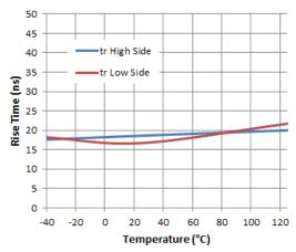
Figure 9. Rise Time vs. Temperature
