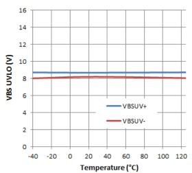
Figure 25. VBS UVLO vs. Temperature
