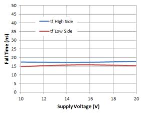
Figure 10. Fall Time vs. Supply Voltage
