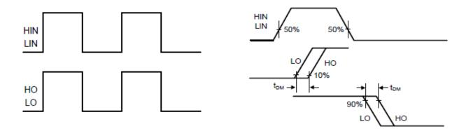
Figure 1. Input / Output Timing Diagram
