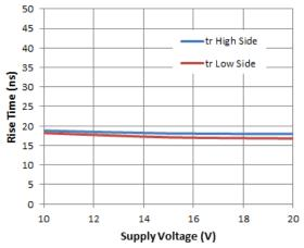
Figure 8. Rise Time vs. Supply Voltage
