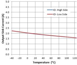
Figure 19. Output Sink Current vs. Temperature
