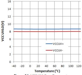
Figure 24. VCC UVLO vs. Temperature
