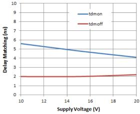
Figure 14. Delay Matching vs. Supply Voltage
