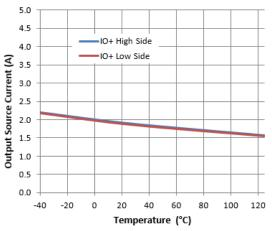
Figure 17. Output Source Current vs. Temperature
