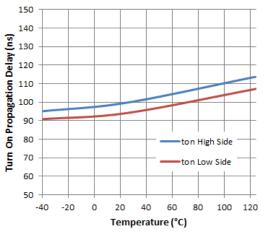
Figure 5. Turn-on Propagation Delay vs. Temperature
