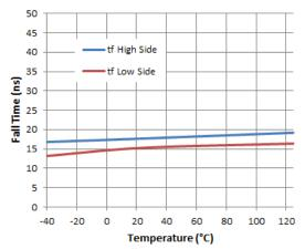
Figure 11. Fall Time vs. Temperature
