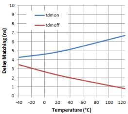
Figure 15. Delay Matching vs. Temperature
